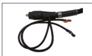
Rotating connection to govern welding wire feeder
