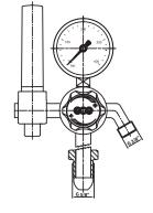
The ECO SAVER keeps a constant level of gas pressure in the downstream system during the welding process. This prevents pressure and flow surges from being created in the system. Surges can create gas wastage and give rise to a poor weld. Weld quality and gas consumption are optimised when the ECO Saver is used as part of the control system.
