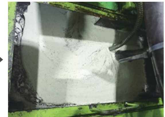
After : Most of aluminum powder and oil floats have been removed.
