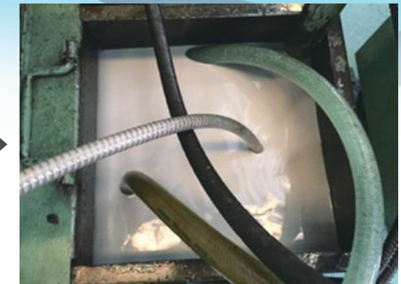
After : Both carbon powder and oil floats have been removed.
