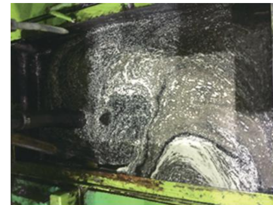
Before : Aluminum powder floats on top of water tank. Tank volume : approx. 500L
