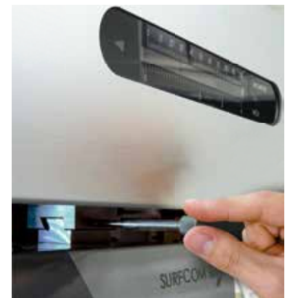
The detector is locked or unlocked by a half turn clockwise or counterclockwise respectively.
