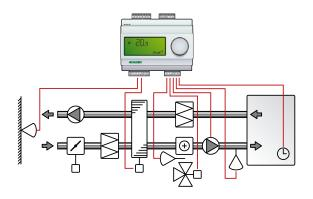
This control mode requires two sensors, "Supply air sensor" on AI1 and "Outdoor sensor" on AI2.
