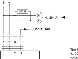
The  $500\Omega$  resistor converts the 4...20mA current signal to a voltage signal DC 2...10V
