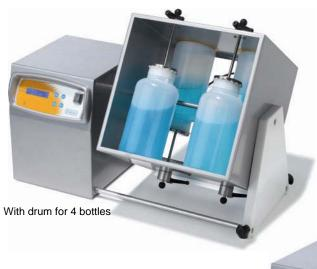
Digital rotary mixer, controlled by microprocessor.
