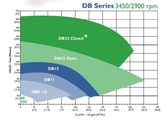
\*Contact the factory for closed impeller DB22 2900 rpm performance. Performances are equal for all other DB models.
