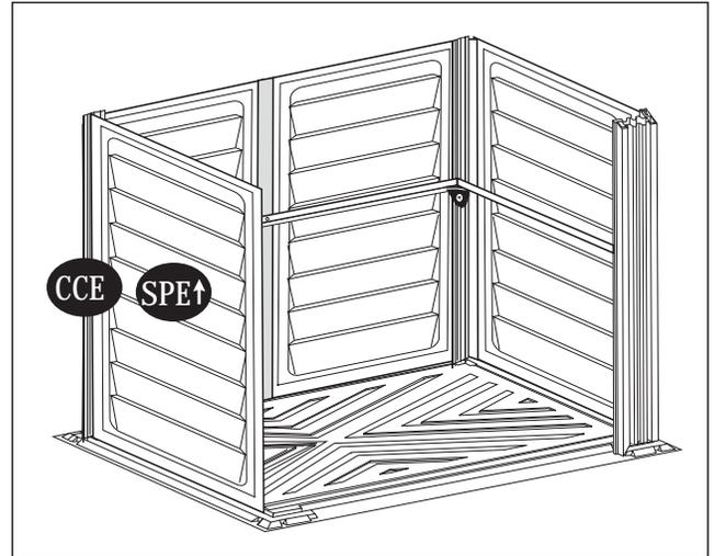
**14.** Slide the front column (FCLE) into the groove of the base pallet (BPF) on the left side of the door. Line up the pre-drilled holes on (FCLE) column with pre-drilled holes on base pallet. Fix with (S5) screws with (S6) washers from outside. See blowup detail.
