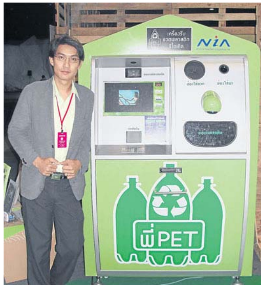
P-Pet's research indicates one machine installed in a community will receive 600-800 bottles per day, totalling 30 kg, according to Mr Angkul.
