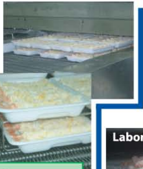
Figure 3 A tray of breaded shrimp in bunches laid on direct in-feed pathway of the tunnel freezer
