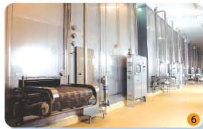
Fully welded stainless steel wall panel enclosure
