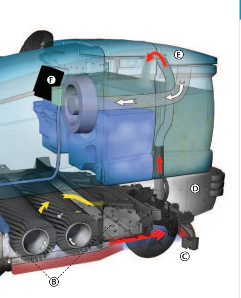
C Maximize water pick-up and reduce maintenance with the Dura-Track<sup>™</sup> squeegee with SmartRelease<sup>™</sup> D Count on durable, steel frame and Grip-n-Go<sup>™</sup> corner rollers to withstand
