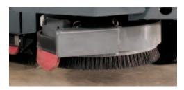
Widen the cleaning path from 40 in/1020 mm up to 54 in/1370 mm Achieve superior edge-cleaning and maximize productivity with an optional side brush.
