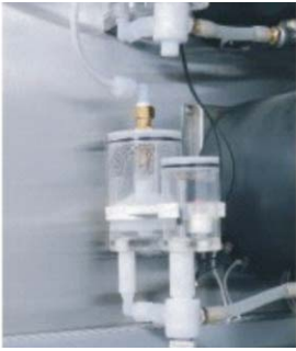
Liquidometer: It controls the height between the humidifier and the wet bulb cup with a power off device when humidifier wants water.
