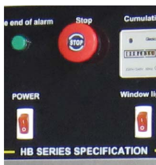
Emergency stop The emergency stop and alarming unit when test finished.
